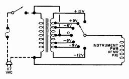
Instruments that are voltage-sensitive must be protected from power-line fluctuations. This circuit does it easily with only a transformer and rotary switch. Addition or subtraction of 12 volts is obtained in 3-volt increments taken from taps on transformer.
